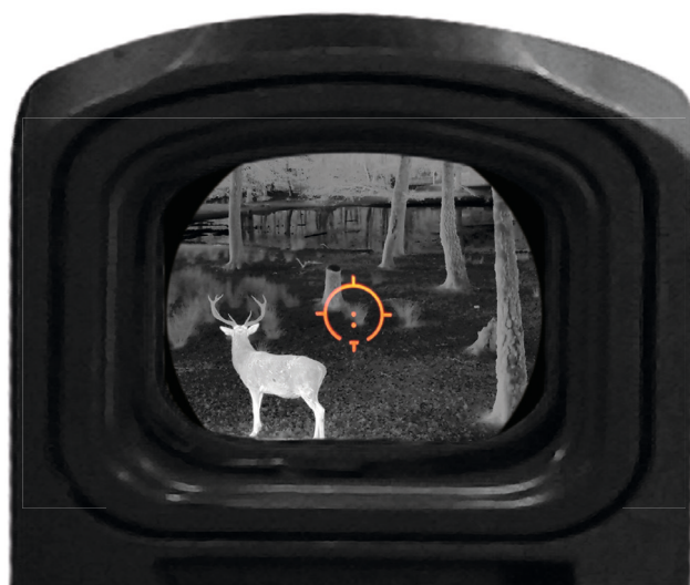
Holosight reticle with thermal image
